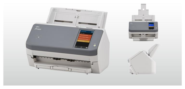
The fi-7300NX boasts a speed of 60 ppm/120 ipm (200/300 dpi) for scanning A4 portraits, loads up to 80 sheets at a time, and ensures utmost efficiency as a standalone scanner that supports both Wi-Fi and ethernet connectivity.
