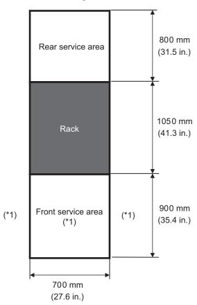
\*1 To mount a chassis on the rack, an area with a depth of 1,200 mm (47.2 in.) is required in front of the rack, and areas with a width of 600 mm (23.6 in.) are required on both the left and right sides of the front service area. If there is a possibility that a chassis will be added later, secure an area with a depth of 1,200 mm (47.2 in.) in front of the rack and areas with a width of 600 mm (23.6 in.) on both the left and right sides of the front service area.
