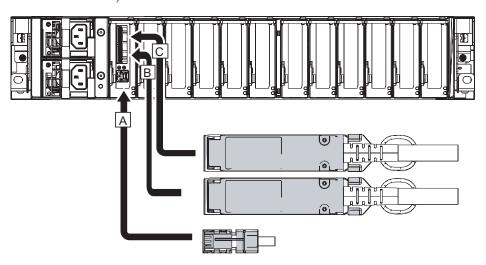
Figure 4-8 Connecting the link cables and management cable (SPARC M10-1 side)
