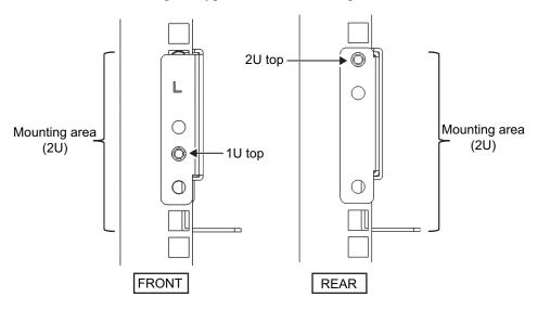
Figure 3-24 Attaching the rail: Fixing location of the screw
