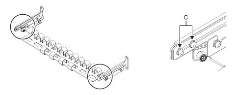
b. Slide the cable support fixing brackets (D in Figure 3-28) to remove them.
