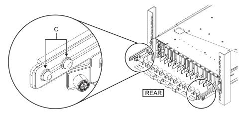
**Note -** If the dimension between the front and rear columns of the rack is less than 740 mm, secure the cable support without sliding it in all the way. The fixing location varies depending on the dimension between the front and rear columns of the rack. Based on Figure 3-38, align the scale marks (E in Figure 3-38) (spacing: 10 mm) on the cable support with the screws (F in Figure 3-38) of the fixing brackets to secure the cable support.
