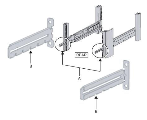
Figure 3-26 Securing the cable support fixing bracket and the rail
