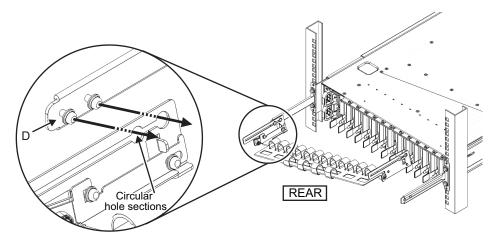
b. Slide in the cable support all the way, and tighten the four screws (C in Figure 3-37).
