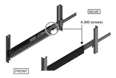
8. Mount the PCI expansion unit in the rack.
