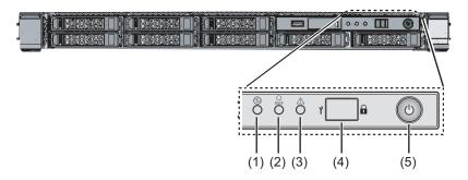
Table 2-12 LEDs and switches on the operation panel
