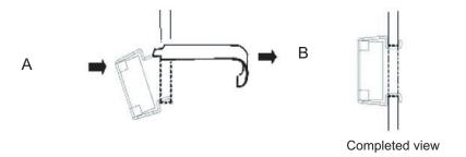
For supporting columns with M6 screw holes
