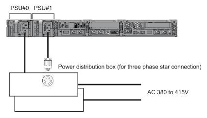
Figure 2-9 Power supply system with three-phase power feed (delta connection)
