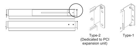
Figure 3-13 Distinguishing the cable supports
