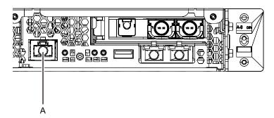
Connect a LAN cable of Category 5 or higher from a GbE port (A in Figure 4-2) to the network switch or hub. The GbE ports are used for the user network. Connect the other servers, other PCs, UPS, etc. that are necessary for business via the network switch or hub.
