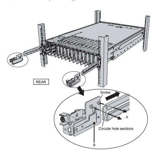
Figure 3-35 Attaching the cable support
