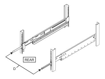
Figure 3-30 Securing the cable support fixing brackets and the rails
