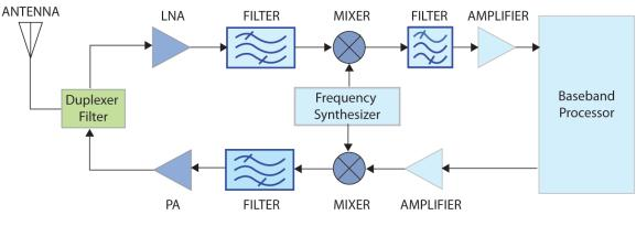
Figure 1 – Simplified RF Transceiver
