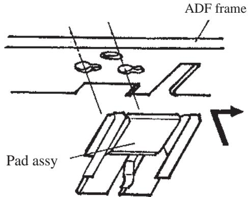
NOTICE: Pad can be replaced by aligning the holes of the pad with the pins of the Pad holder.
