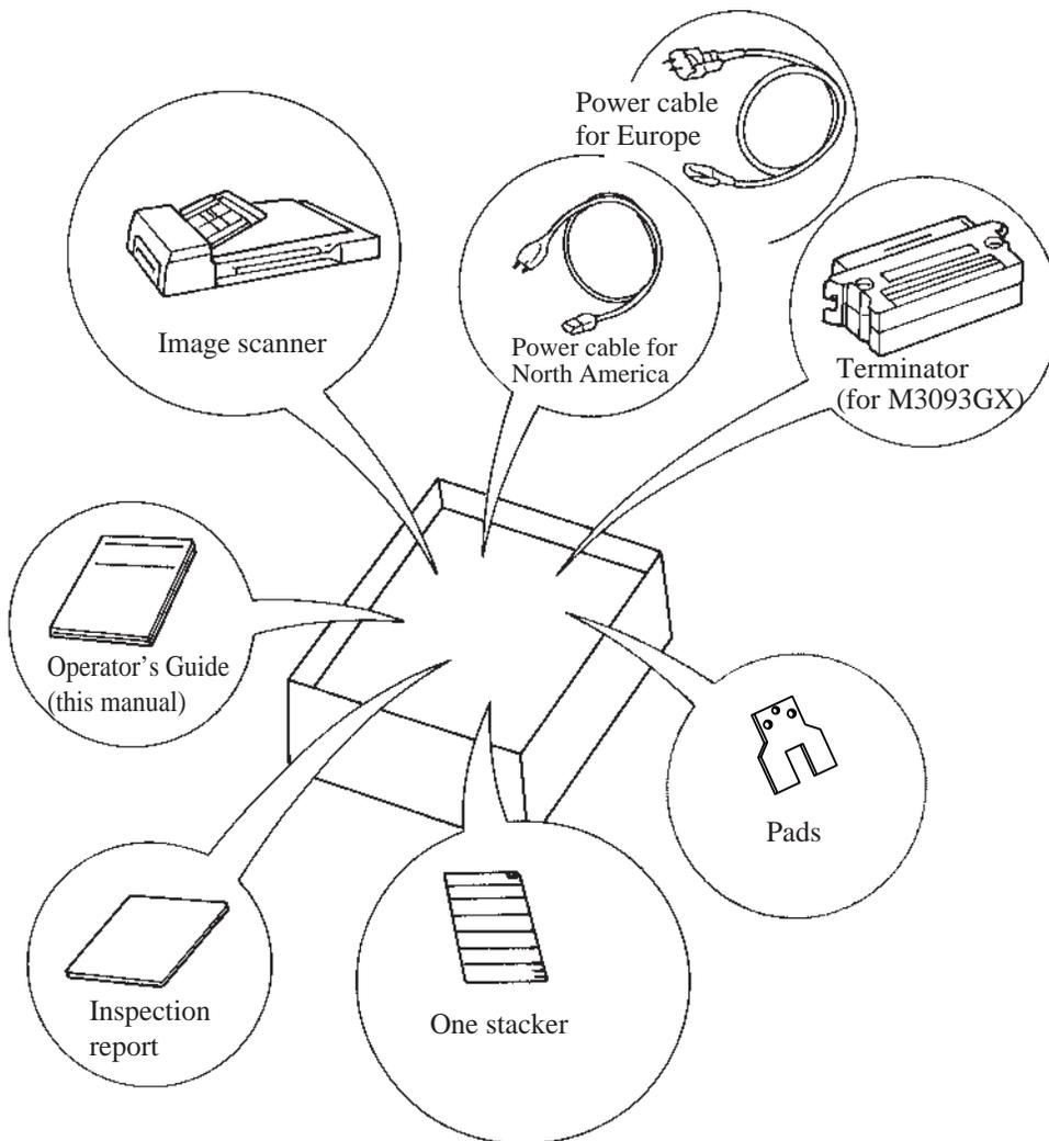
Figure 2.1 Received components
