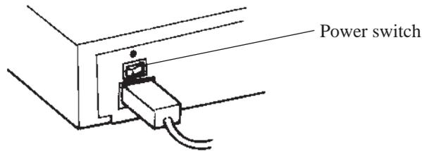
Press “O” on the power switch to turn off the power.
