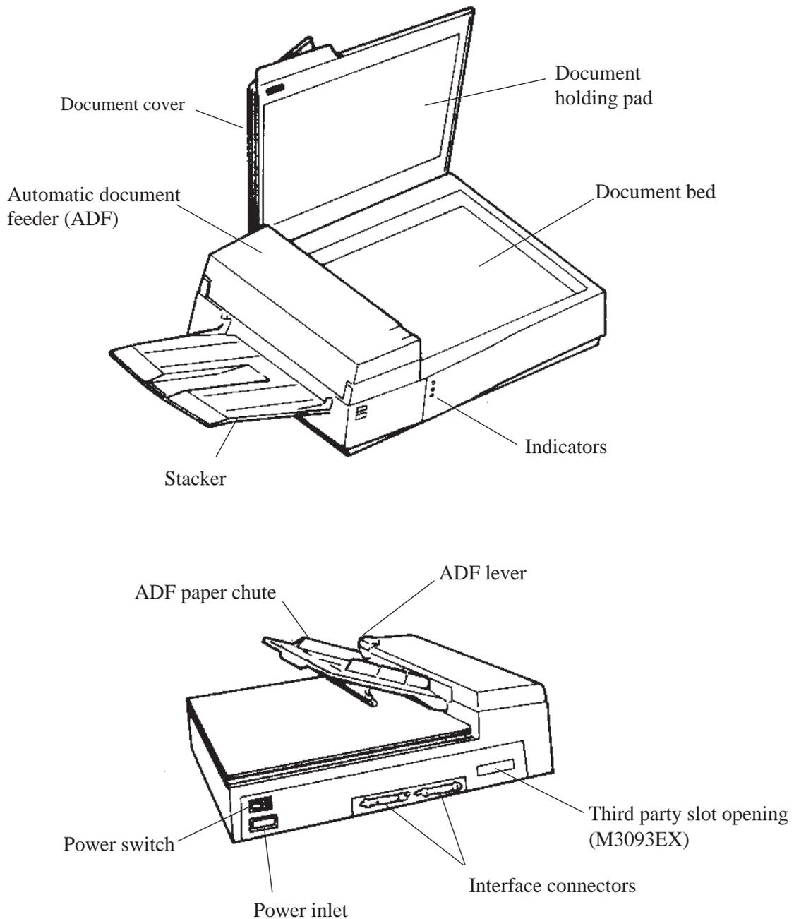
Figure 2.2 M3093EX/GX parts names
