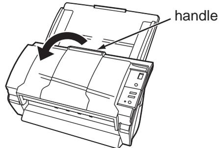
2. Lift the paper stop and swing forward by inserting your fingertips into the indentations on the stacker.
