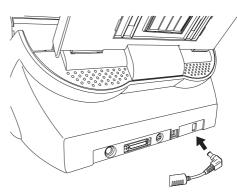
3) Plug the AC cable into the outlet.
