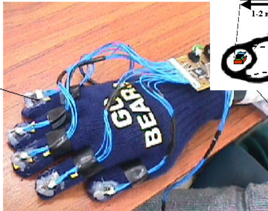
Wrist controller, RF transmitter and battery pack
