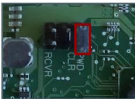
Fig. 2: Jumper in Password Clear position
