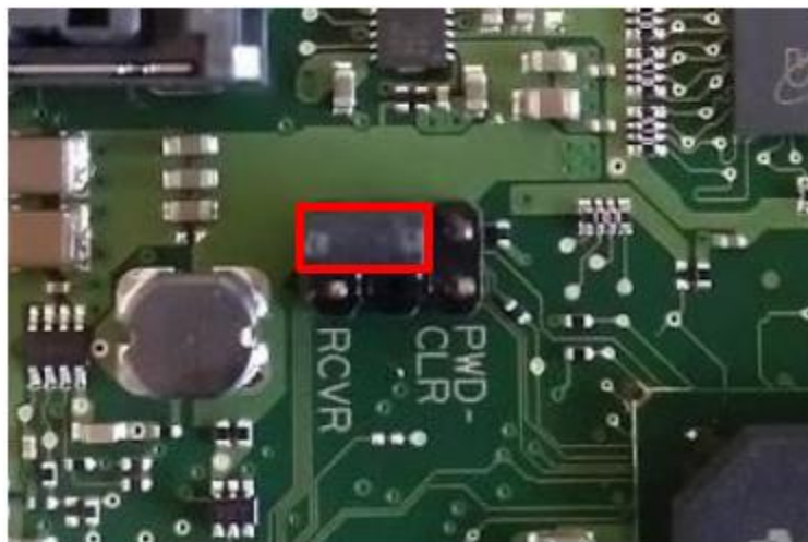
Fig. 1: Jumper in neutral position
