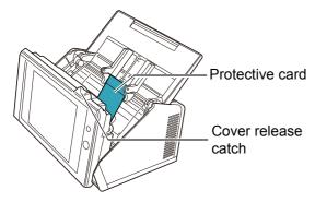
**4.** Pull the stacker forward, and then remove the tape and protective card.
