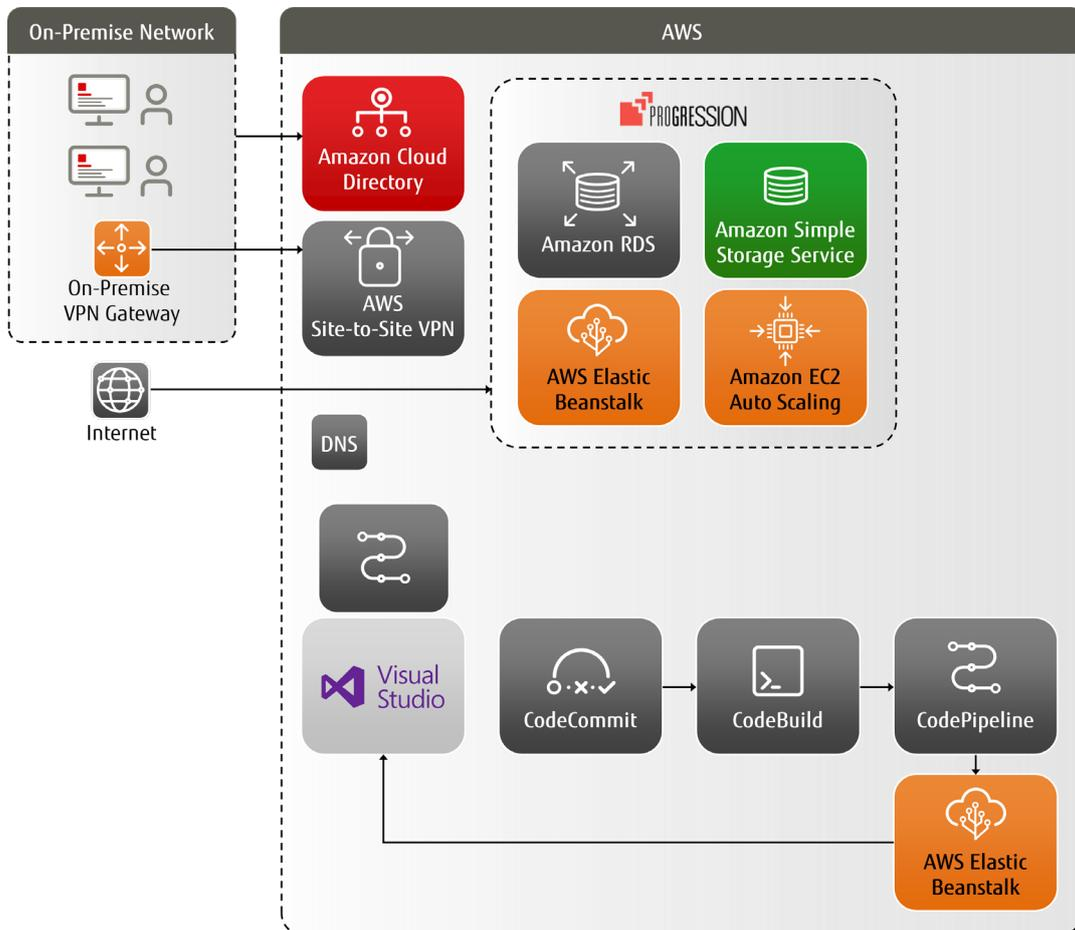
Figure 8 - AWS Deployment solution stack
