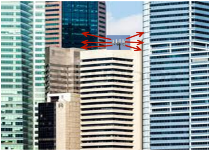
Figure 7: DL interference from macrocell to femtocells near windows can be severe.
