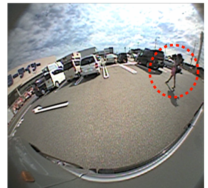
Sample showing the driver's view of the video images. Note the pedestrian behind the automobile is clearly visible to the driver.
