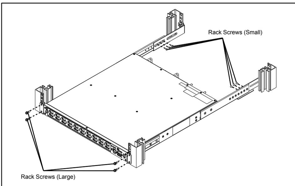
2. Slide the XG2000 forward, and remove it from the rack.
