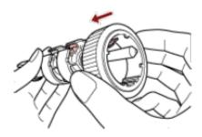
b. Insert the retaining clip of the other pick roller into the slot.
