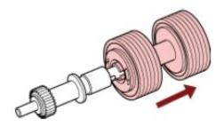
6. Attach a new brake roller on the shaft. Insert the protrusion on the shaft into the slot.
