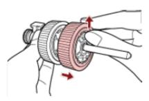
b. Pull out the other pick roller from the shaft as you lift the retaining clip.
