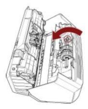
c. Hold the bushing on the shaft to lift up the shaft end, pull the other shaft end out of the slot, and then lift up the pick roller to remove it.
