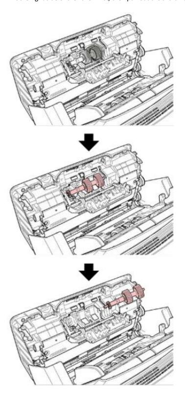
5. Remove the brake roller From Its shaft.
