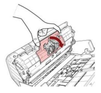
b. Lift the right side of the roller First, then pull out the shaft from the slot on the left.
