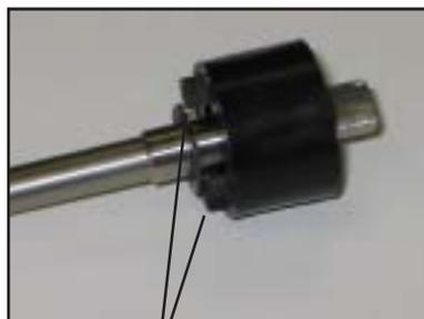
Tabs in Brake Roller Shaft
