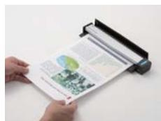
Re-insert the page without pressing the Scan button to scan the other side.
