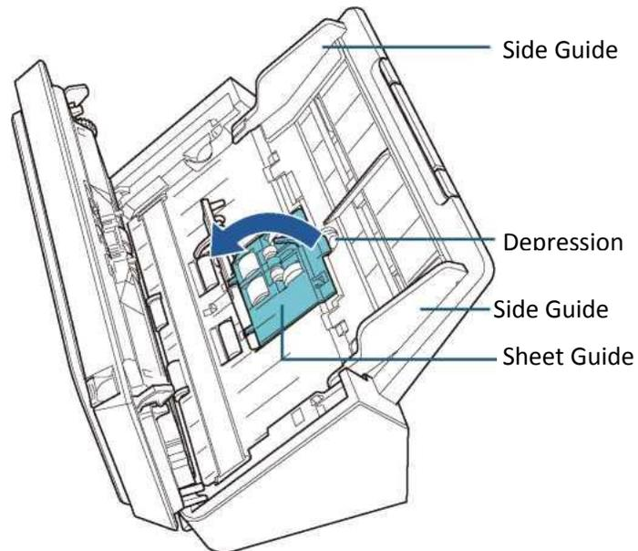
b. Slide the pick roller and remove it from the top.
