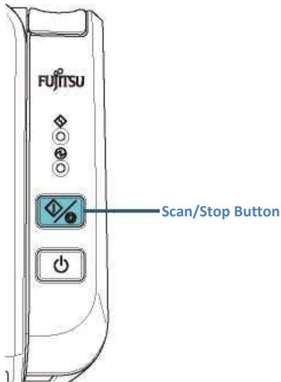
Put a piece of cloth moistened with Cleaner F1 or a sheet of Cleaning Wipe against the roller surface, and wipe horizontally. Wipe the whole surface by pressing the scan/stop button to rotate the rollers.
