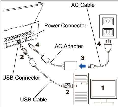
3. Connect the AC cable to the AC adapter (hereinafter called the "power cable").
