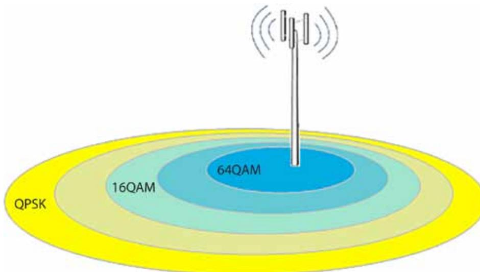
**Figure 4: Adaptive Modulation**
