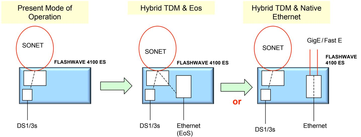
**Figure 10: FLASHWAVE 4100 Extension Shelf Ethernet Options**
