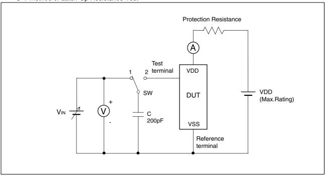
Note Charge voltage alternately switching 1 and 2 approximately 2 sec interval. This switching process is considered as one cycle.
