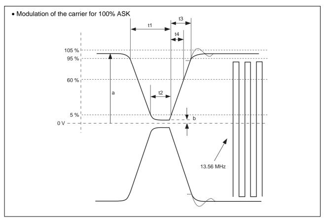
Maximum and minimum values of t1, t2, t3 and t4 are shown in the table of " **E**RECOMMENDED OPERATING CONDITIONS". In this table, y is 0.05 (a-b) and the maximum value of hf and hr is 0.1(a-b).
