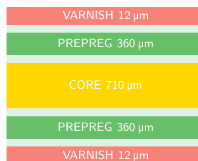
Figure 26: Recommended PCB stackup
