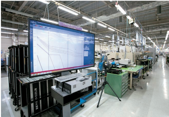
The data visualized in VisualLine can be checked at large displays attached to the lines
