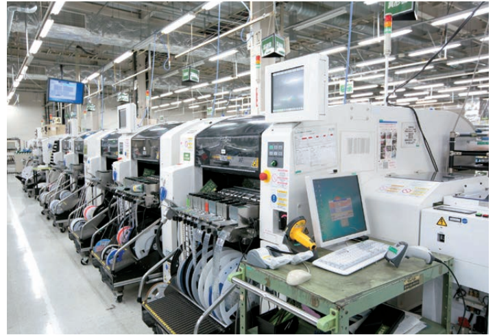
The printed circuit board (PCB) mounting lines at the Yamanashi factory, where IoT was introduced
