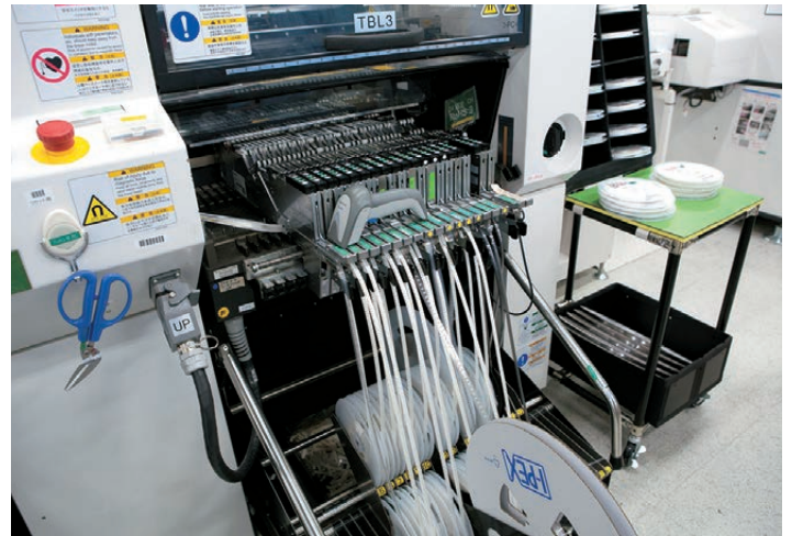
When it seemed like a line would run out of parts, replacements were placed by the surface mounting machine (the reels on the right-hand stand). This shortened the amount of stoppage time due to parts replacement
