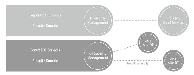
A key best practice is network zoning or segmentation: logically separating enterprise IT from operations IT and introducing sub-zoning to control the access of one location from another and from one OT device to another. This approach is applied both in the central data centre and in the outlying facilities.
