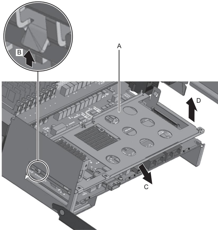
7. Remove the one black screw (A in the figure) fixing the center part of the radiator on the front side and the four screws fixing the CPU memory unit board (B in the figure).
