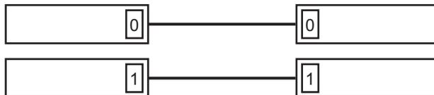
Figure 8-38 Label position of link cable (electrical)
