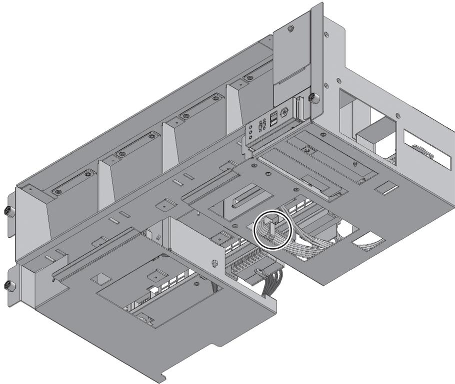
5. **Support the fan shelf from the bottom with one hand and insert it carefully into the cabinet.**
