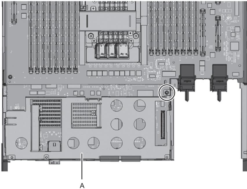
6. Lift up the left projecting lever of the XSCF mount (A in the figure) by fingers about 2 mm (0.1 in.) (B in the figure) and slide it to the front about 8 mm (0.4 in.) (C in the figure). Then, remove it upward (D in the figure).
