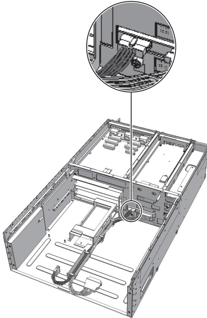
9. **Remove the cable from the clamps.**
