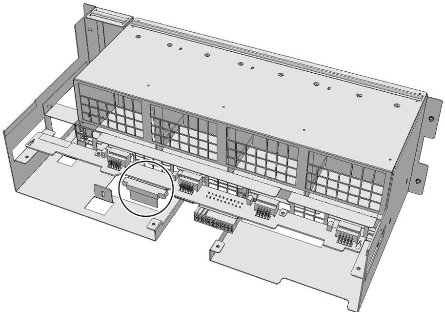
9. Remove the cable connecting the fan shelf and operation panel from the
