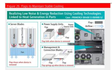
At the same time, Fujitsu optimizes cooling fan cycles in accordance with the ambient temperature and heat generated by internal chips. This measure minimizes power consumption for cooling based on current heat and system load.
