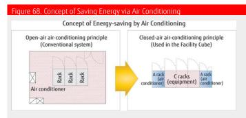
For the cooling unit of S Type and M Type, Fujitsu adopted a sensible heat system that reduces heat generated by devices without unnecessarily dehumidifying the interior. This system leads to excellent cooling efficiency compared with conventional air conditioning. In addition, because air flows only inside the Facility Cube, it is highly dust resistant and quiet during operation.
