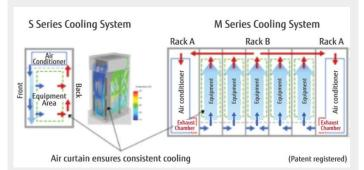
This flow of air down the front of the Facility Cube becomes an air curtain, so administrators can open the front door and work on the ICT equipment inside. During maintenance, the air curtain is so effective that administrators are rarely disrupted by temperature alerts that commonly occur in other products, even where air conditioning is installed in the rack. Fujitsu's smart design enables work to be performed without powering down the unit.
