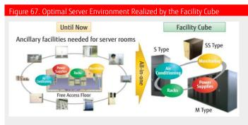
Until now, the principle of cooling in server rooms has been based on cooling the entire space with open-air systems. The Facility Cube is a closed, airtight environment that has its own system for cooling only the rack itself. This concept realized extensive energy savings.
