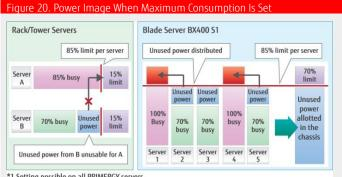
\*1 Setting possible on all PRIMERGY servers \*2 Set absolute value of allowable usage (I.e., 850W for a 1,000W server at 85% limit)
