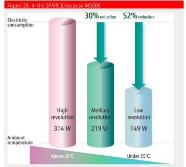
In storage, fan rotation is controlled in 10 stages. At high temperatures, fan speed is raised immediately to enhance cooling effectiveness. What's more, Fujitsu has realized fan operation at a comparatively quiet 40 decibels (dB).
