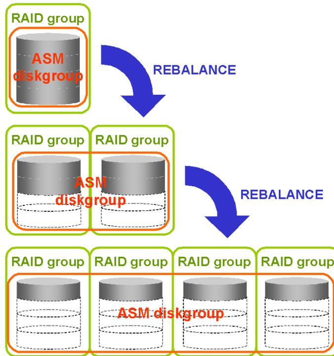
Figure 18 ASM disk addition and data rebalancing
