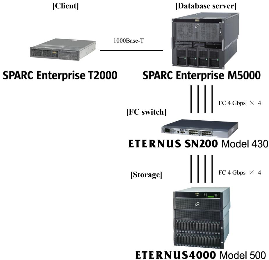
Figure 2 Schematics of system configuration
