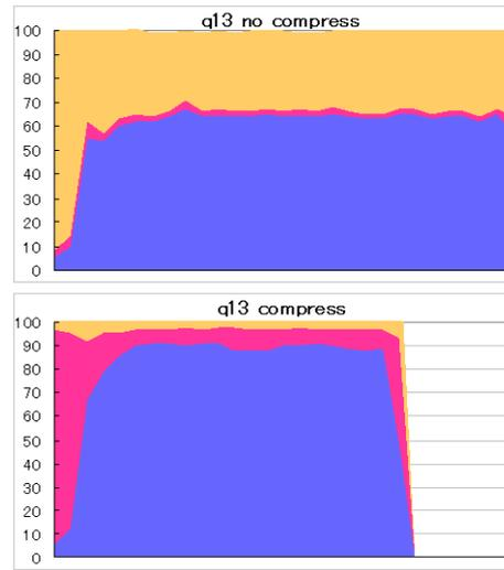
**Figure 15** Temporal changes in CPU use during execution of q13 (top: non-compressed, bottom: compressed)
