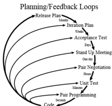
図：Planning and feedback loops in extreme programming
