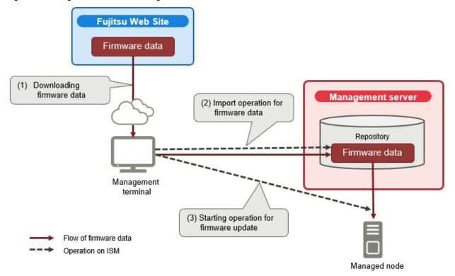
This section describes the procedure from firmware data preparation to the execution of the firmware update for the PRIMERGY BIOS/ iRMC.
