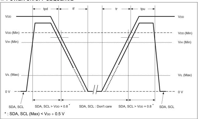
When applying relatively short term  $V_{DD}$  pulse whose peak is more than 1.7V, it is required to set falling time, tf more than 0.4ms/V. (In case  $V_{DD}$  rises over 1.7V and falls just after that, if this term is short, device may lose its function.)
