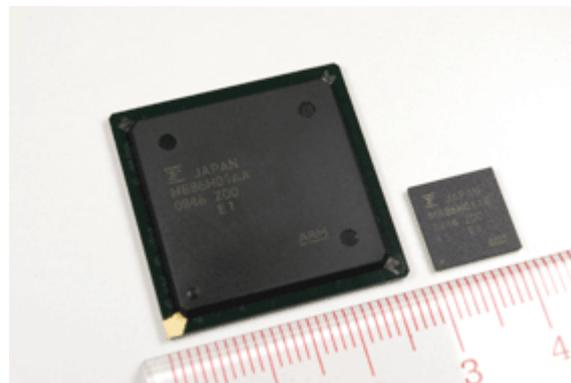
Figure 1: SD multi-decoder LSI, MB86H01
