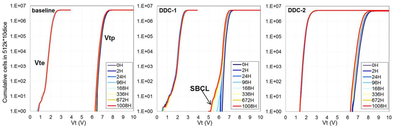
Fig.15: Vte & Vtp distribution after 1k cycling & 150C bake
