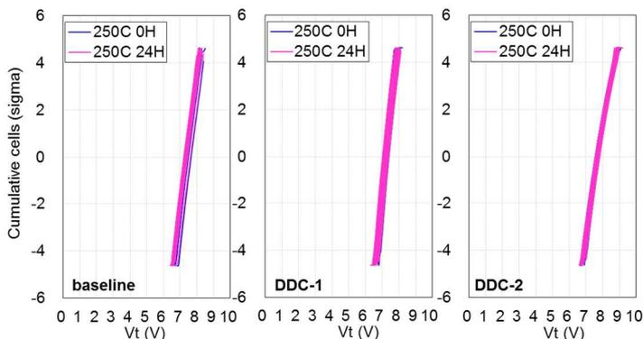
Fig.13: Vtp before & after 250C bake for 512k\*70dice
