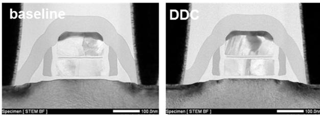
Fig.4: a) X-TEM of flash parallel to BL on baseline & DDC
