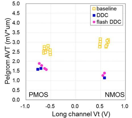
Fig.6: Pelgrom AVT as a function of long channel  $V_T$
