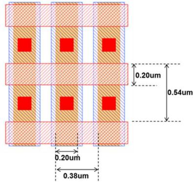
Fig.2 FLOTOX flash cell layout
