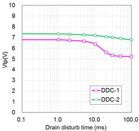
Fig.11: Dependence of Vtp shift on DD time
