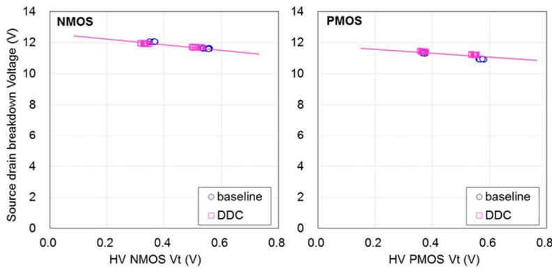
Fig.7: a) BV of HV NMOS b) BV of HV PMOS
