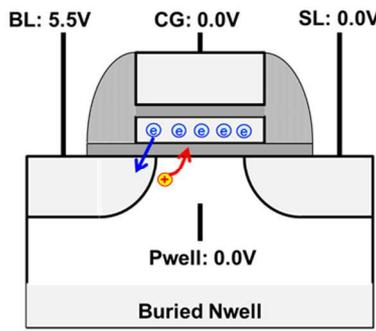
Fig.9: Bias condition of DD
