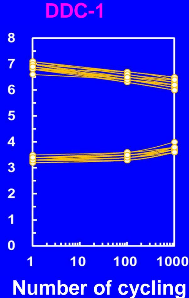
512k (512WL\*1024BL) macro , 20 dice(10 for  $V_{te}$ , 10for  $V_{tp}$ ) , 150C bake
