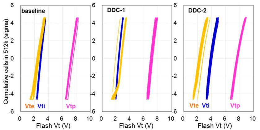
Fig.12: Distribution of UV, Vtp & Vte in 512k\*70 dice
