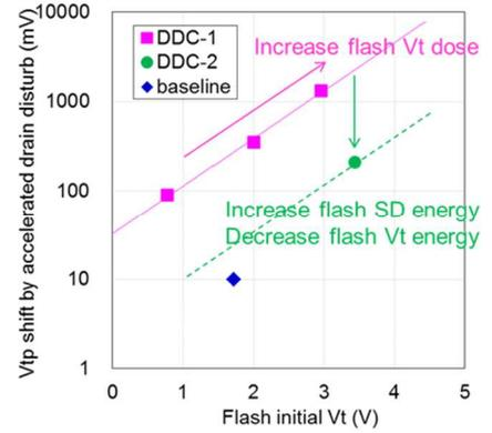
Fig.10: dependence of Vtp shift by DD on Vti
