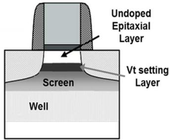
Fig.1 Structure of DDC transistor
