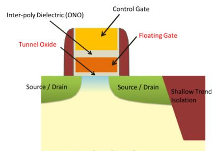
**Fig.1 FLOTOX Structure**
