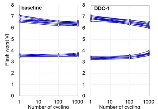
Fig.14: flash window as a function of cycling
