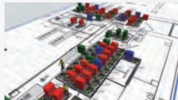
3D simulation of the ATM production line.
