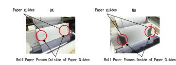
■Attention 10) When adjusting the position of the paper guides, the position on the same line as the holder is used as the reference. Be careful not to be outside the reference Also, adjust the position so that it is within 10mm inside
