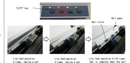
■Attention 6) By holding down the "LF/FF" switch, the form feed operation is performed and the roll paper is feed forward about 550 mm. Therefore, do not hold down the "LF/FF" switch. If you performed form feed operation, turn the paper feed knob counterclockwise to eject the roll paper and start over from 3-1
