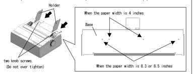
Attach the holder temporary about in the position shown below
