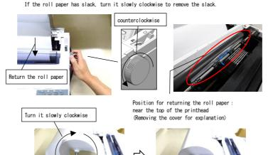
3-6. Press the "LF/FF" key on the printer operation panel to perform line feed operation. Repeat pressing the "LF/FF" key until the bail roller close and holds the roll paper (The approximate number of times to press down is  $5 \sim 10$ .)
