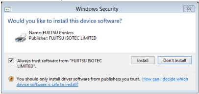
4. Connect the printer to the computer and switch on the printer. When the printer power on, it will install the DL3100 driver automatically. When the installation is finished, click "ok".
