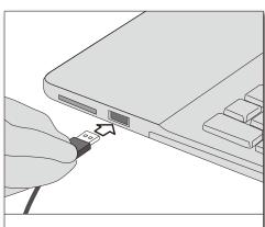
**2.** Connect the printer and PC by USB interface
