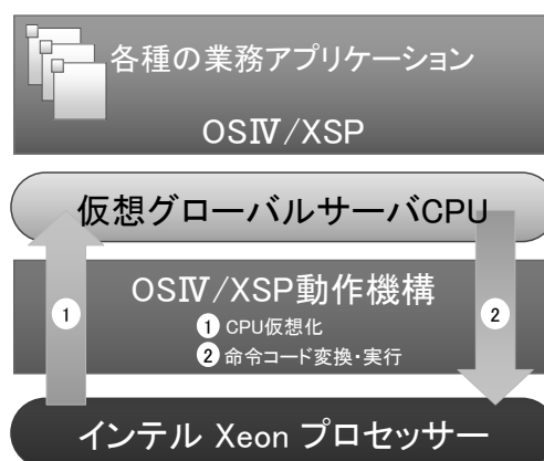
図-10 OSIV/XSP動作機構の概念 Fig.10-OSIV/XSP translation facility.
