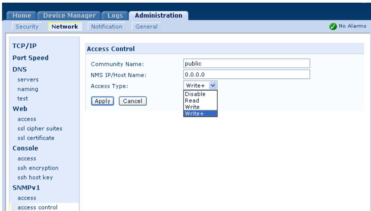
図9. Switched Rack Mount PDU SNMP v1 Access Control 設定画面
