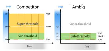
**SPOT™** Patented SPOT Platform dramatically reduces an internal operating voltage to 0.5V, and reduce energy usage to 1/5 upto 1/10 than the other competitors.
