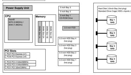
\*Components installed as standard configuration marked in grey.
