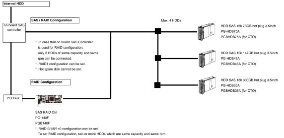
should be connected to on board SAS Controller.
