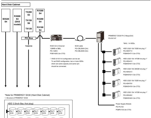
When more than 7 internal HDDs are installed in PRIMERGY SX30, 2 SCSI Cables must be connected with 2 channels for RAID Controllers.
