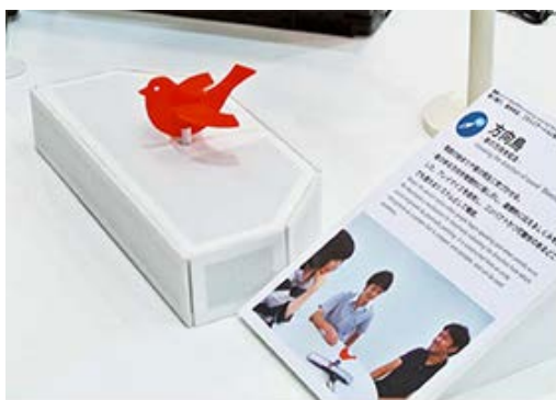
Hoko Dori device shows the direction from which a sound came
