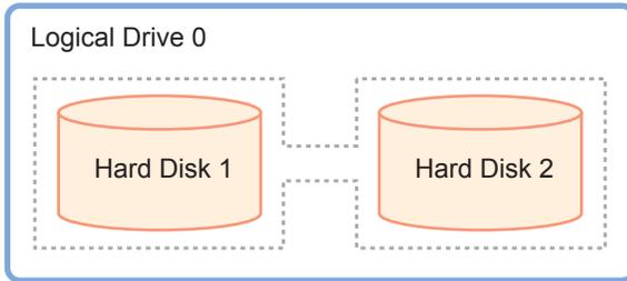
As for the status of the logical drive, "Online" represents the normal state, "Critical" means a state where one hard disk unit has a failure and the redundancy feature is inactive, and "Offline" means a state where both of hard disk units have failures and the logical drive is inactive.
