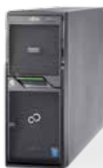
2-way tower server PRIMERGY TX300 S8
