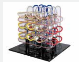
High-dimensional torus interconnect structure
