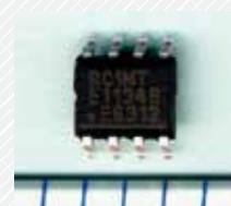
I²C interface 1 megabit FRAM "MB85RC1MT"
