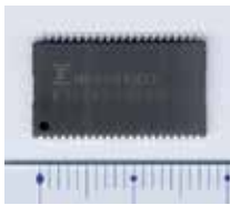
4 Mbit FRAM non-volatile memory compatible with SRAM MB85R4M2T
