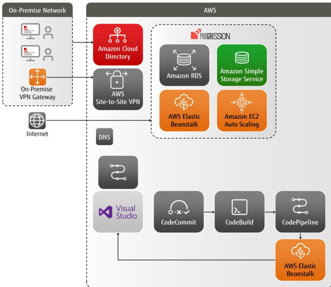
Figure 8 - AWS Deployment solution stack
