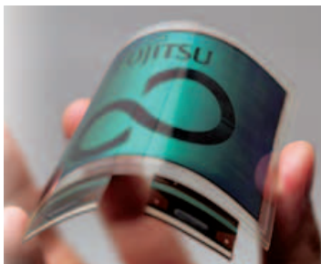
Bendable display using a flexible substrate
