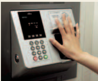
Palm vein authentication access control unit
